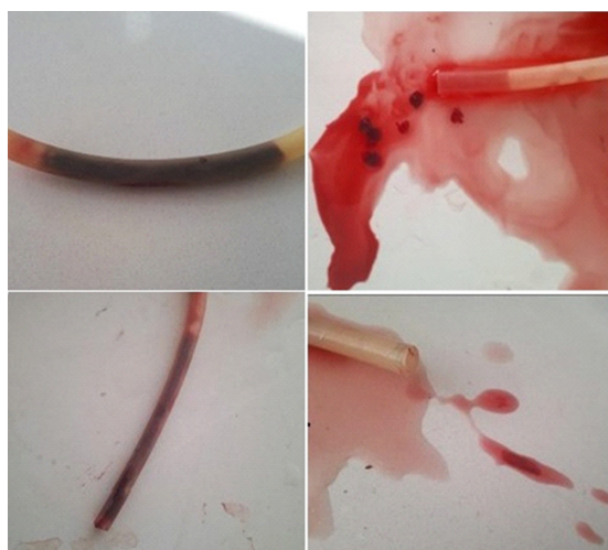
Figure 12: Compressed Samples. Images (Left) show a pair of 10-minute-old venous blood clots having formed within a rubber tubing sized to resemble a coronary artery. Images (Right) show the resultant clots flushed
